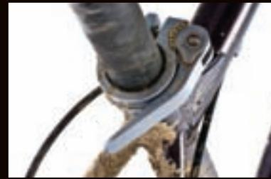
Chromag's Seat QR uses a large piece of brass under the cam to help reduce friction—no shredding weird shims or washers here. It was smooth, secure and noise-free. You can't ask for much more from a quick release.
